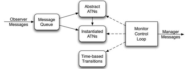
**Figure 3: Overview of the monitor control loop.**
