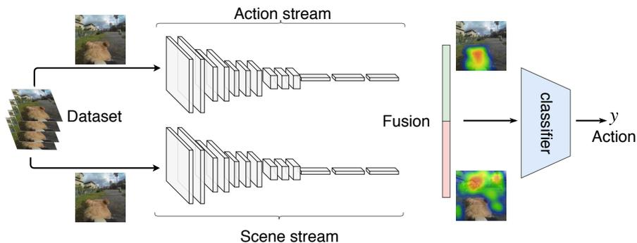
**Fig. 1.** Two-stream architecture composed by a stream to recognize actions and a stream to recognize the context scene with a late fusion.
